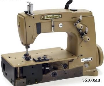
These new 56100s are distinguished from their predecessors by a new bearing for the left mainshaft. This replaces the bushing used in earlier styles. The new bearing handles the load stress at that crucial point much more effectively than a bushing. The bearing allows the shaft to run smoother and cooler. No more downtime or repair labor due to a burned up bushing!
